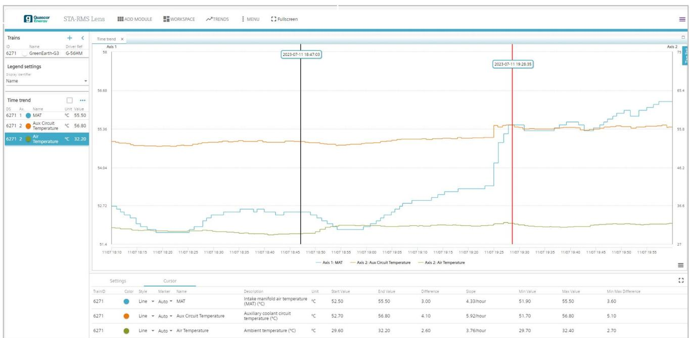
Auxiliary water circuit temperature and MAT (intake manifold temperature) reaction after dry cooler set point increase
